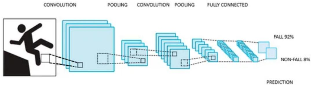
**Figure 2.** Typical convolutional neural network (CNN) architecture.
