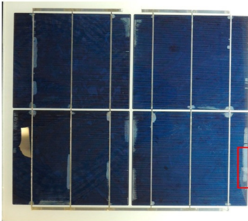
Figure 4. Four cells initially stressed at 85 °C/85% RH, 1000 h for DH test, and then biased at (–1000 V) for 292 (the area covered by the rectangle used for SEM and EDS analyses). Adapted with permission from ref. [34]. Copyright 2018, Elsevier.
