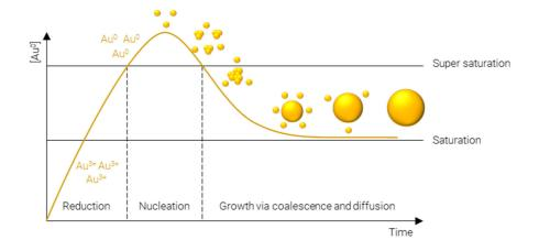
Figure 1. LaMer model of metal nanoparticle formation.
