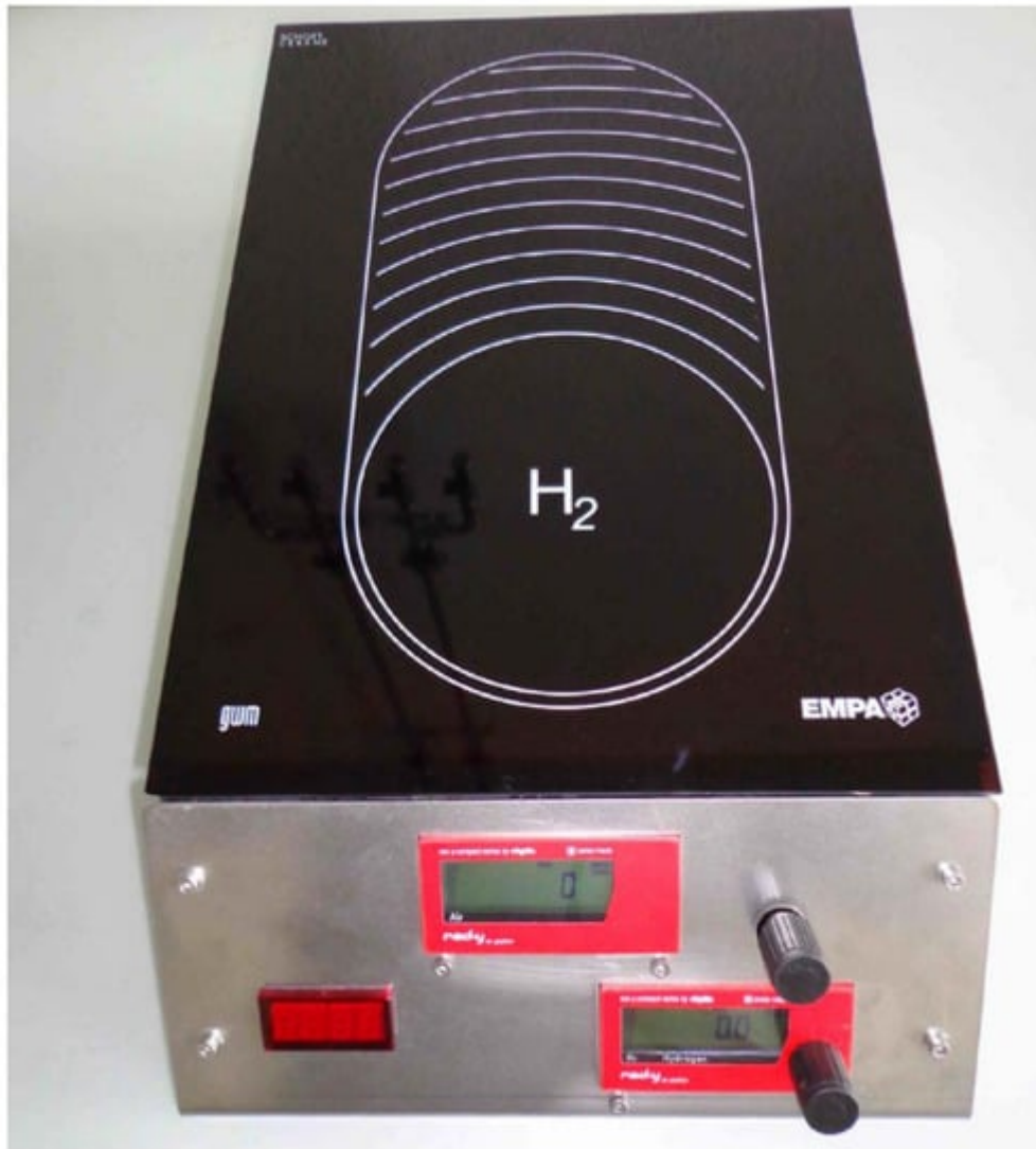
Figure 4. Assembled catalytic hydrogen combustion cooker [91] (reused with permission from Elsevier).
