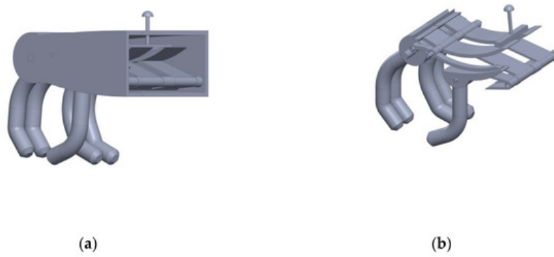
Figure 1. Initial 3D computer-aided design (CAD) reconstruction of the first “Iron Hand” of Götz von Berlichingen. (a) General view of the artificial prosthetic hand; (b) view after virtual removal of the chassis with insight into the mechanics.
