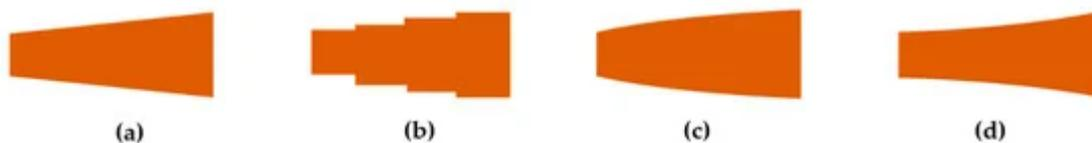
**Figure 2.** Schematic of the (a) linear; (b) multi-sectional; (c) parabolic; and (d) exponential Si inverse tapers (top view).
