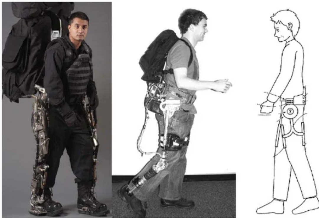
Figure 2. BLEEX Exoskeleton (left) [15] , the quasi-passive exoskeleton (center) [16] , and the “Motion Assisting Device” [17] .
