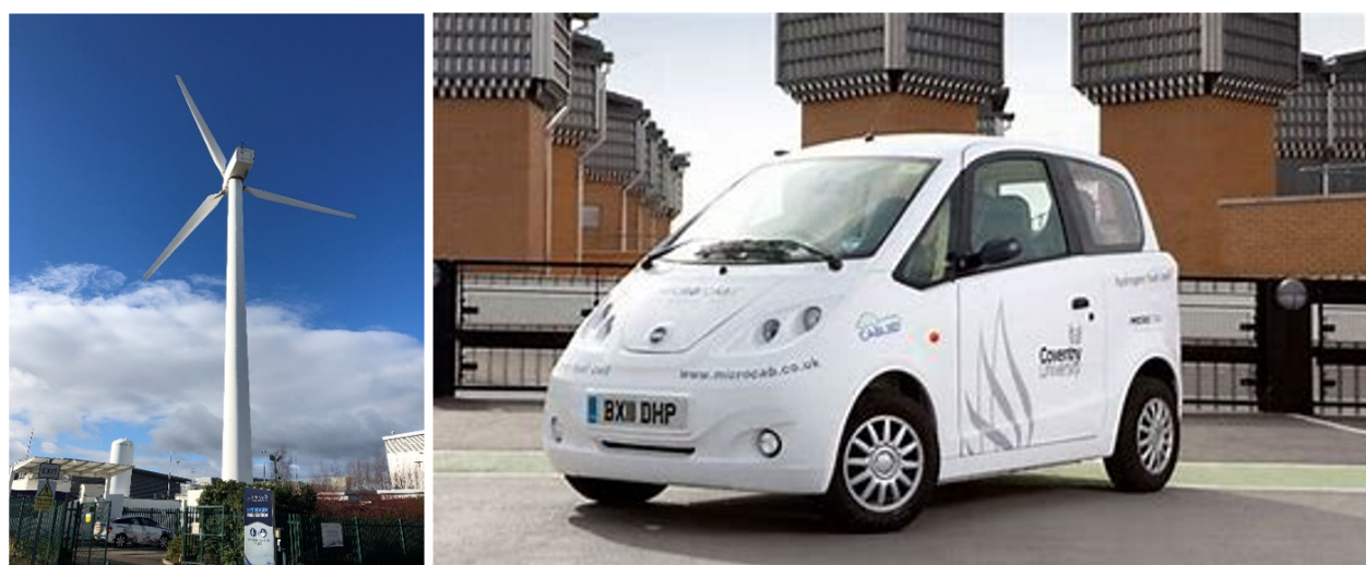
Figure 6. left: Rotherham hydrogen station based on wind turbine electrolysis; right: Microcab for taxi fleet to utilise the hydrogen asset.
