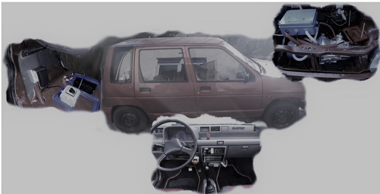
Figure 1. Laboratory production of EV Daewoo Tico with the AGM battery pack.
