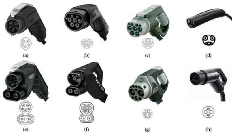
Figure 2. Types of electric vehicle plugs [16][17][18][19][20] : (a) Type 1; (b) Type 2; (c) GB/T (AC); (d) Tesla inlet (USA); (e) CCS 1; (f) CCS 2; (g) GB/T (DC); (h) CHadeMO.
