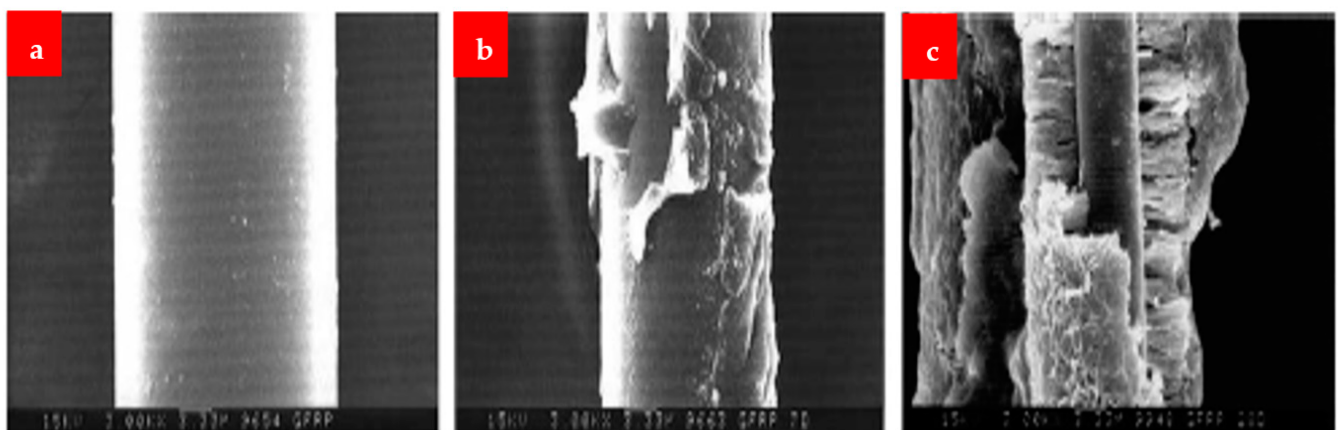
Figure 13. GF (a) normal, (b) 7 days under NaOH and (c) 28 days under NaOH [30].
