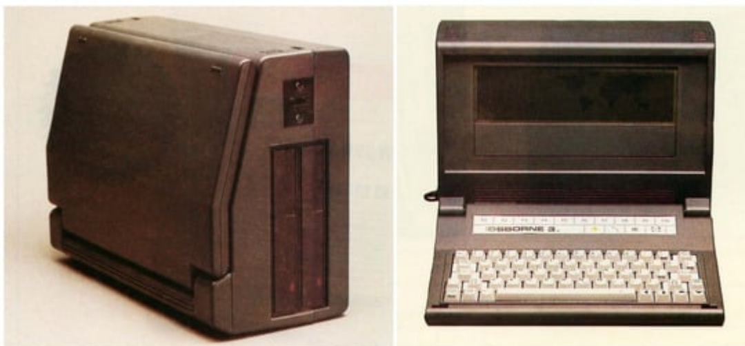
Figure 5. The Osborne 3 with an 80-character by 16-line liquid-crystal display (LCD) and two 5.25" floppy-disk drives. Source: Internet Archive (1985) [16] .
