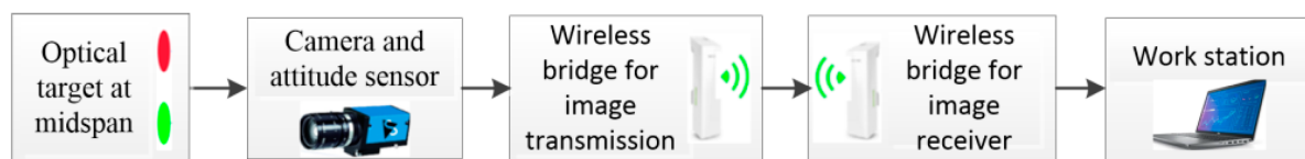
Figure 4. Vision-based system for relative sag measurement.
