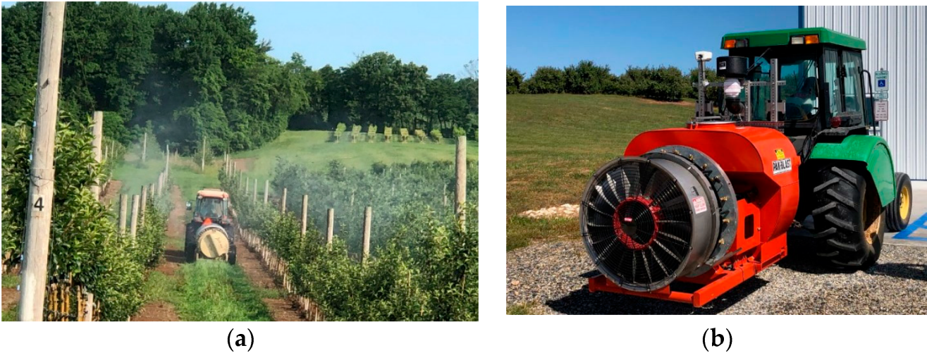
Figure 1. Air blast spraying systems (a) constant rate air blast sprayer; (b) intelligent sprayer.
