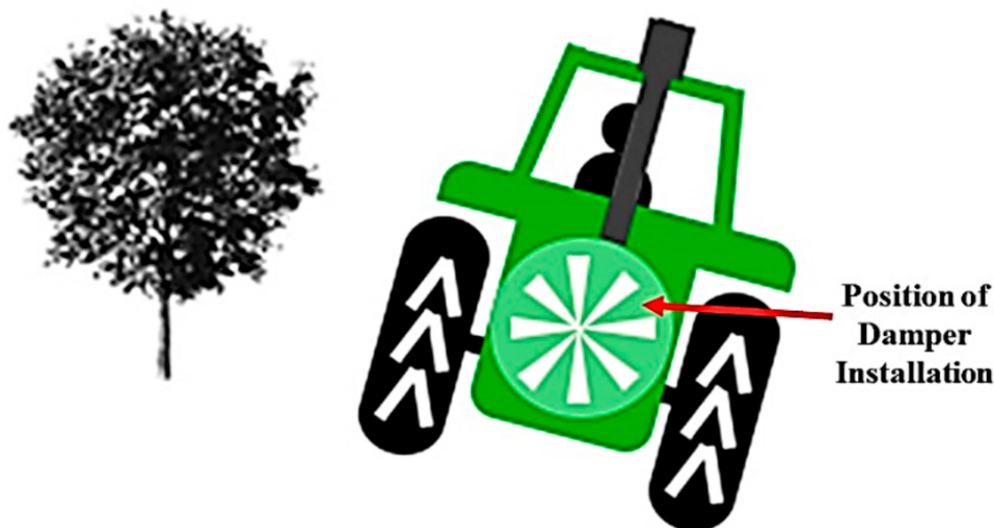
Figure 2. Position of damper installation for precision sprayer airflow control.
