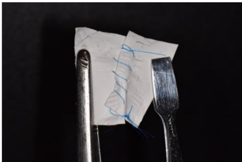
Figure 2. Nanofibre-based membrane obtained after 60 min of ELS with the following parameters: PCL 12% w/v in DCM/DMF 7:3, 17 kV potential, 27 G needle, 0.6 mL/h of flow rate. Nikon D3500, macro 105 Sigma tamron lens, Sigma ring flash. See the mechanical resistance during stretching the same membrane of Figure 5 after cut then sutured with 5/0 polypropylene.
