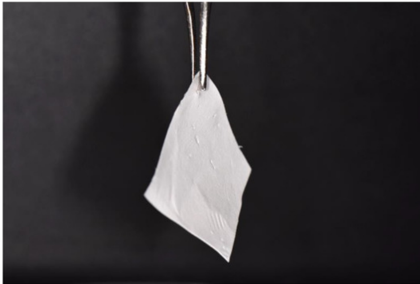
Figure 1. Nanofibre-based membrane obtained after 60 min of ELS with the following parameters: PCL 12% w/v in DCM/DMF 7:3, 17 kV potential, 27 G needle, 0.6 mL/h of flow rate. Nikon D3500, macro 105 Sigma tamron lens, Sigma ring flash. Membranes can be handled easily with surgical tweezers.
