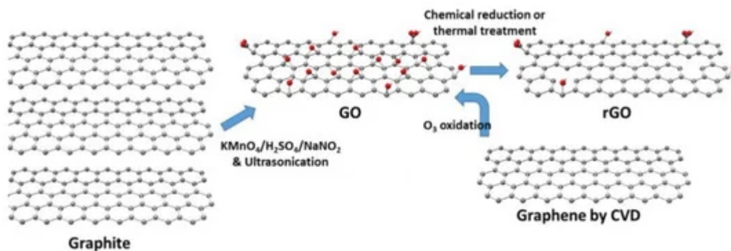
Figure 4. Structure and preparation of GO and rGO [44].
