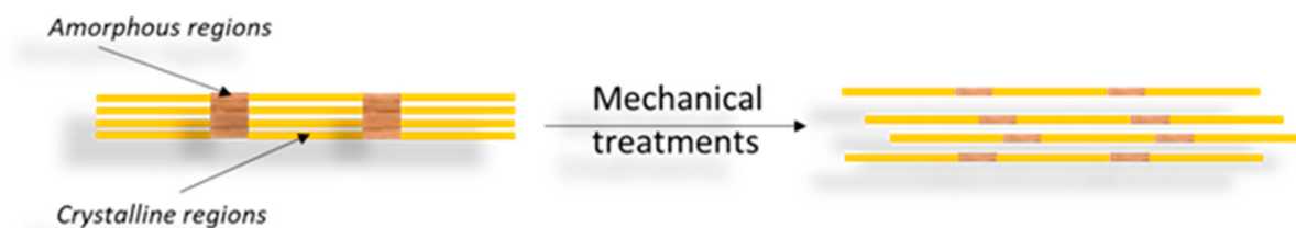
Figure 2. Scheme for obtaining CNFs through a mechanical process of cleaving the cellulose fiber to the nanometric size.
