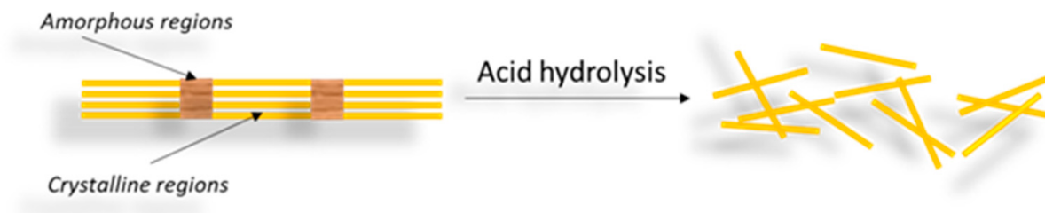
Figure 1. Scheme for obtaining CNCs by acid hydrolysis of cellulose, with the removal of the amorphous region and leaving only the crystalline region.
