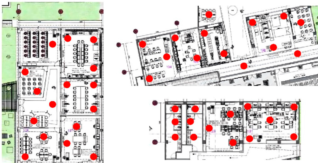
Figure 2. The BLE devices (red dots) were located at several locations of the rooms of the CEDETEC buildings.
