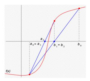
The first two iterations of the false position method. The red curve shows the function f and the blue lines are the secants. https://handwiki.org/wiki/index.php?curid=2076972 The convergence rate of the bisection method could possibly be improved by using a different solution estimate.
