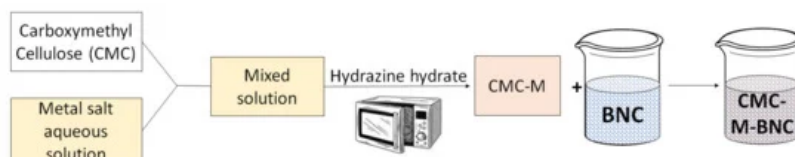
Scheme 1. Preparation of the colloidal carboxymethyl cellulose (CMC)-M nanoparticles and carboxymethyl cellulose (CMC)-M-BNC dip-catalyst.
