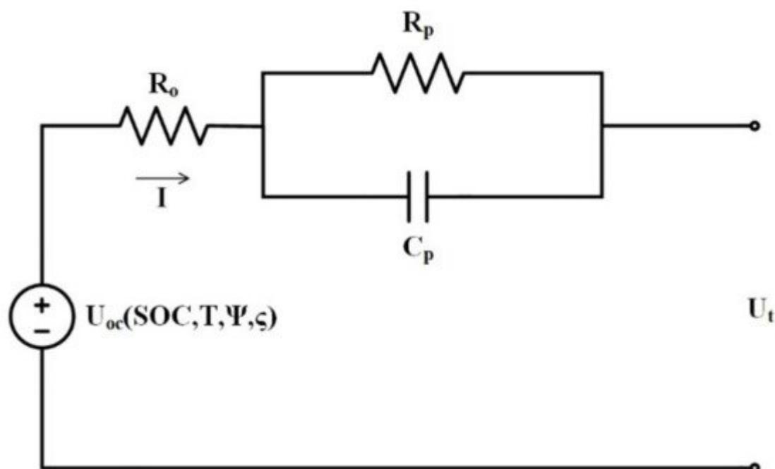
**Figure 11.** 1-RC model with multi-dependent OCV [16].
