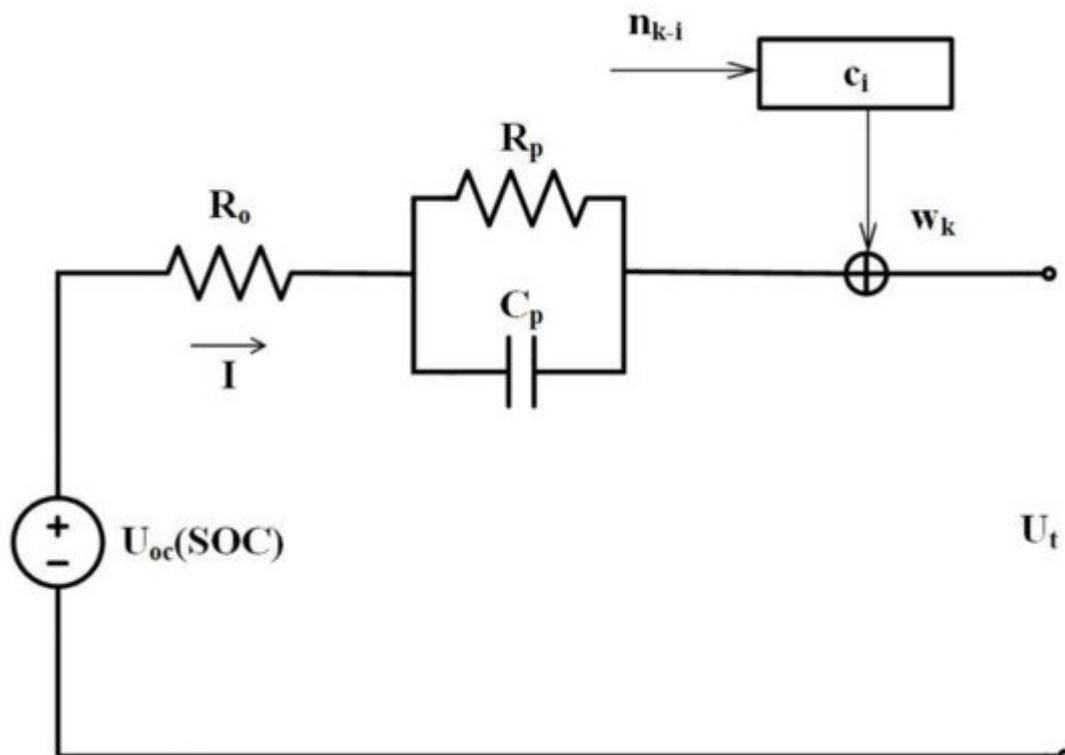
**Figure 8.** 1-RC model with a moving average noise [12].
