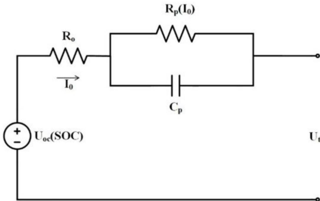
**Figure 9.** 1-RC model incorporating Butler–Volmer equation [13][14].
