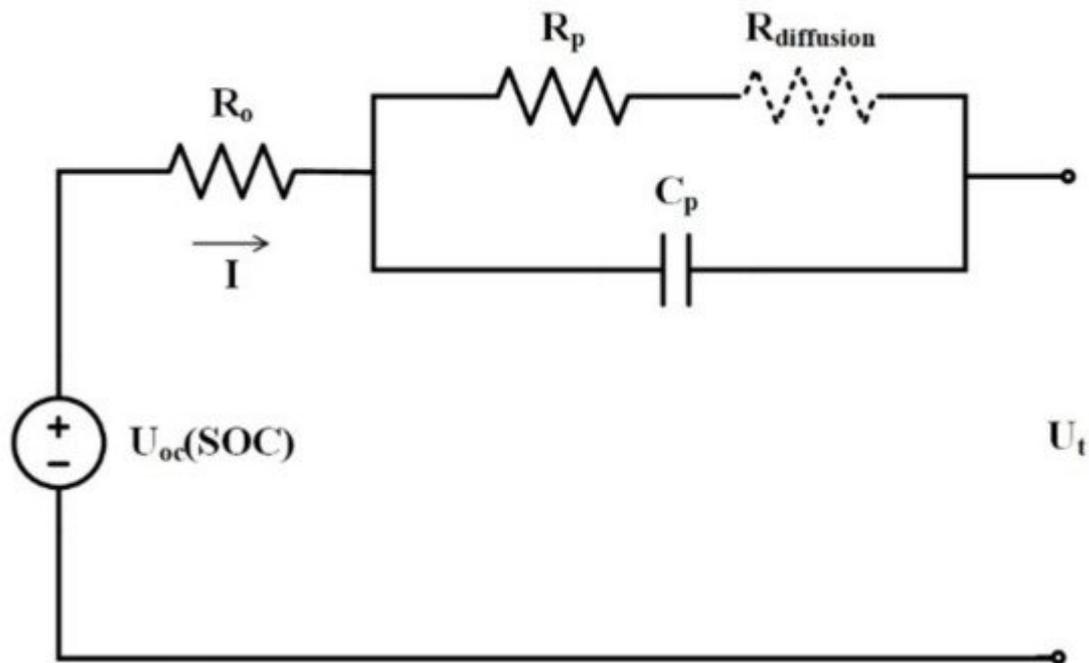
Figure 5. 1-RC model with diffusion resistance [5].
