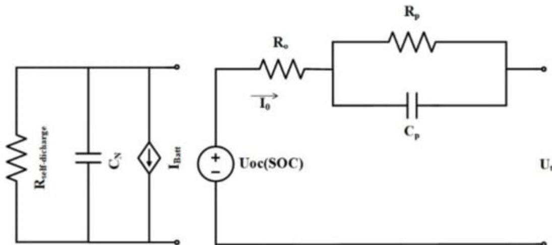
**Figure 7.** 1-RC model considering self-discharge phenomenon [11].
