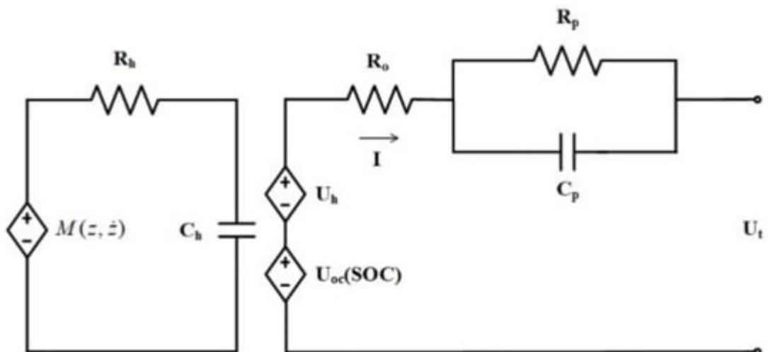
**Figure 6.** 1-RC model with one-state hysteresis [6][7][8][9].
