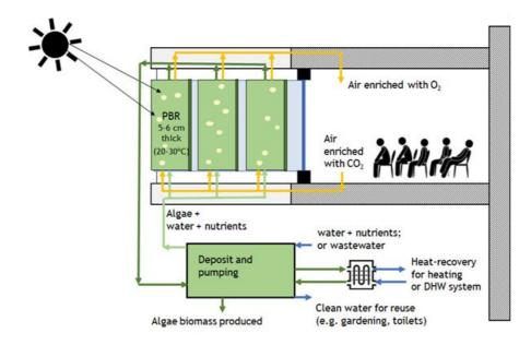
Microalgae cultivation system integrated into a building as the proposed solution for indoor air treatment, showing the air flow in and out of a room (authors' own creation).
