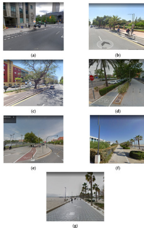
Figure 2. Types of bike lanes: (a) bicycle lane, (b) protected bike lane, (c) sidepath on median, (d) sidepath with vegetated curb, (e) sidepath without curb, (f) bike track, and (g) cycle path [16][17] .
