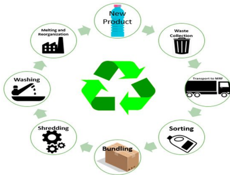
Figure 1. The typical stages involved in plastic recycling.
