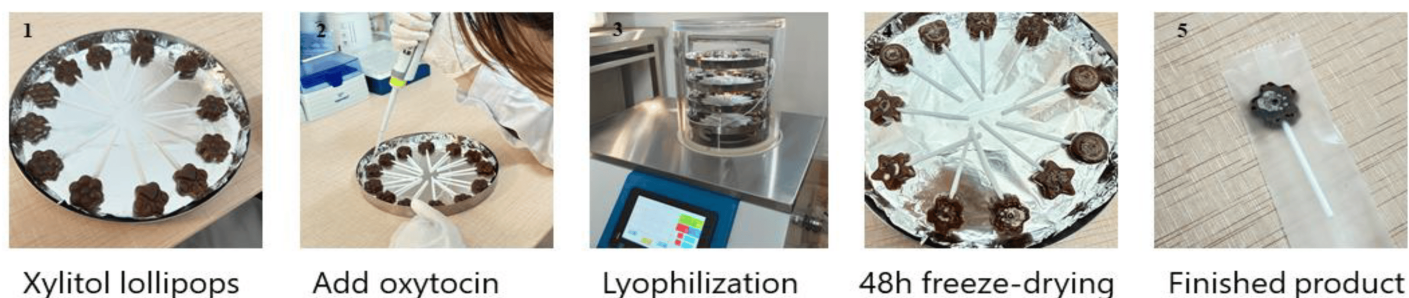
Figure 2. Method (left to right) for producing sugar-free (xylitol) lollipop candies with oxytocin acetate (OXT) freeze-dried on one surface of the lollipop ('oxipops').
