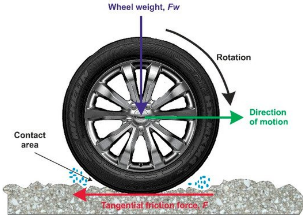
Figure 3. Typical sketch of forces acting on a rotating wheel (concept taken from [5][15]).
