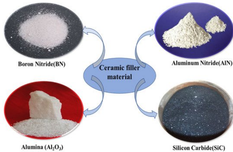
Figure 3. Commonly used thermally conductive ceramics filler.
