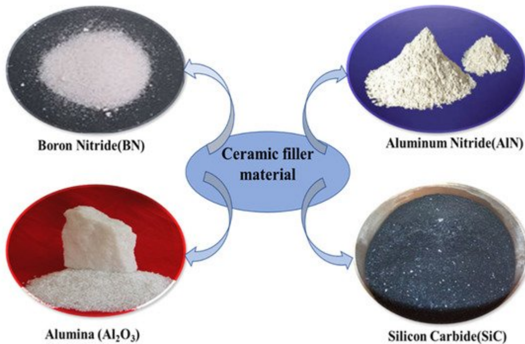
Figure 3. Commonly used thermally conductive ceramics filler.
