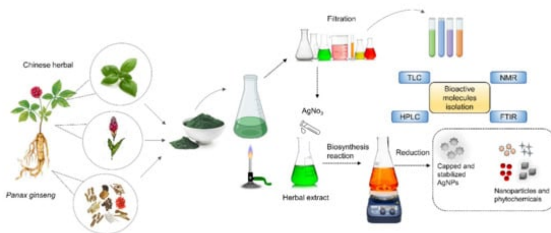
Figure 1. Biological synthesis of silver nanoparticles (AgNPs) from Chinese herbs containing bioactive molecules.
