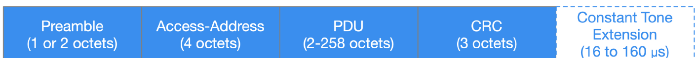
Figure 3. Structure of a Bluetooth 5.1 packet with the duration and position of the CTE. Associated apps add CTE
