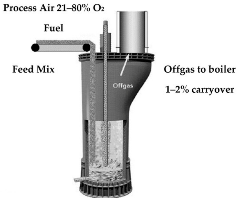
Figure 1. Scheme of Isasmelt technology [10] .
