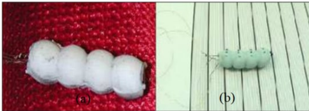
Figure 17. View of robotic earthworm design using shape memory alloy locomotion technology (a) with and (b) without micro-legs [21].
