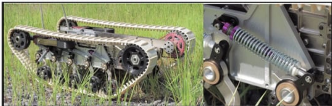
Figure 7. The spring-loaded suspension between tank track drives and supports [11] .
