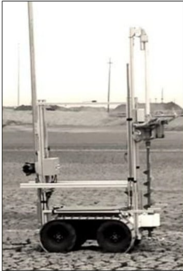
Figure 8. Researchers equip a Husky UGV from Clearpath Robotics with tank tracks that fit over the original UGV wheels [8].
