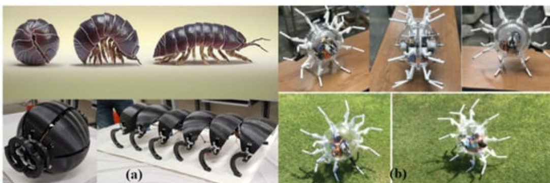
Figure 21. View of (a) rolling isopod-based robot demonstrating the conglobation process [26] and (b) golden-wheel-inspired rolling robot [16].
