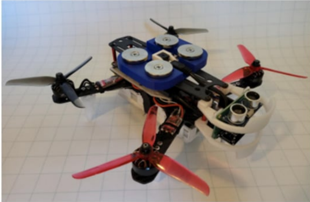
Figure 32. Semi-autonomous precision-docking quadcopter constructed from a racing drone frame with custom sensors and flight controllers [42] .
