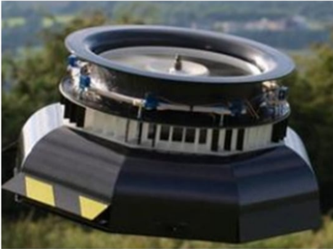
Figure 28. Aesir drone utilizing a single rotor and the Coandă effect for flight [38].
