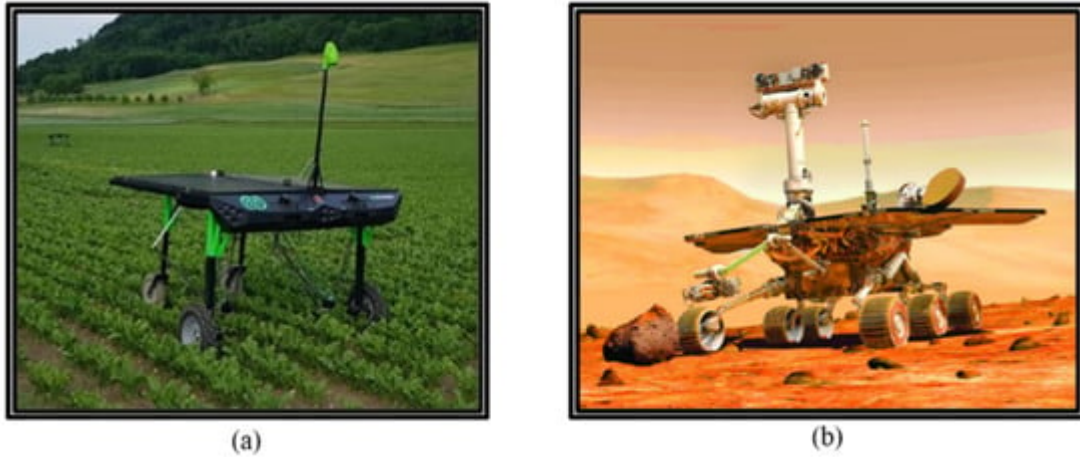
Figure 2. Examples of wheeled UGVs with specialized functionalities: (a) four-wheeled UGV drives through seedlings, picking weeds between rows [5]; (b) six-wheeled UGV traverses Mars' surface.
