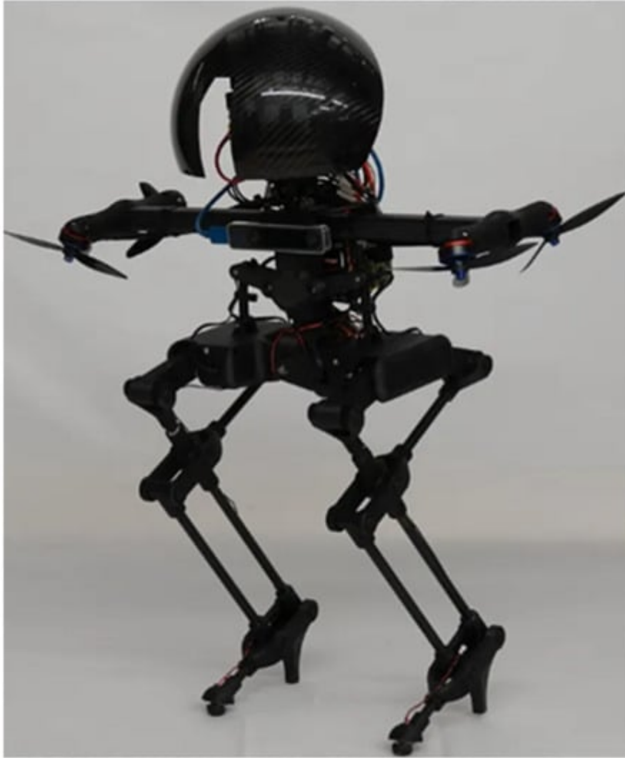
Figure 40. LEONARDO, the walking, hopping, flying drone, is modeled after birds that can both fly and hop in order to navigate telephone lines [68] .
