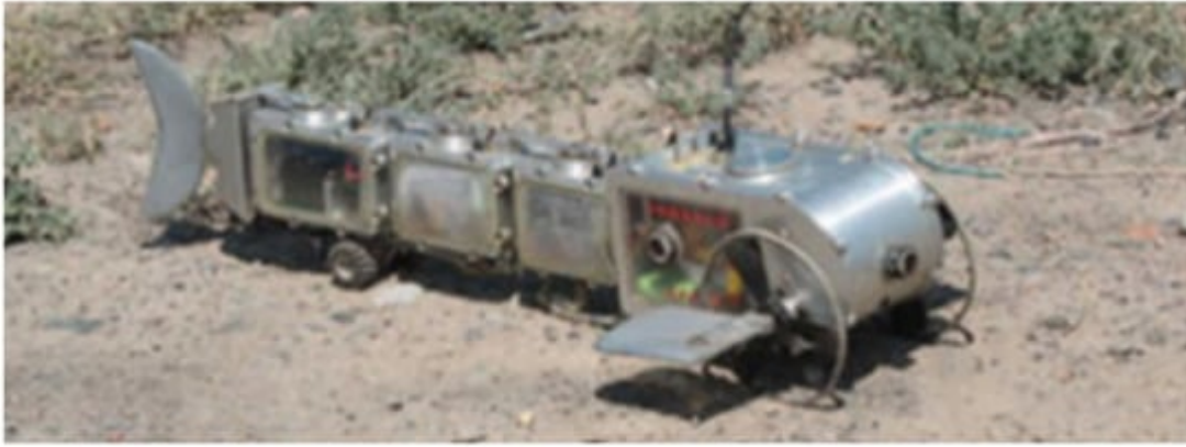
Figure 23. Mechanism design of AmphiRobot-II; prototype of the amphibious robot in the field test [28].
