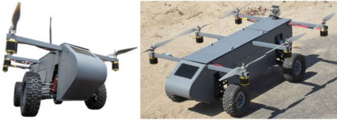
Figure 43. Advanced Tactics Panther Drone is one of the first unmanned ground vehicles (UGVs) capable of flight in addition to terrestrial travel. The UGV uses four powered wheels, as well as four rotors that act as a quadcopter with pitch and roll control [73].
