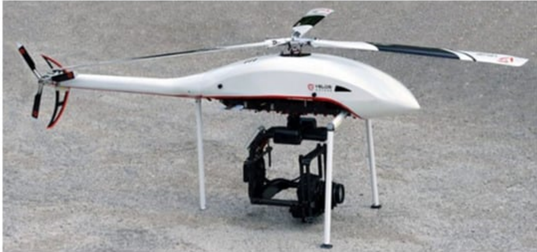
Figure 24. Single-rotor helicopter-style drone used for surveillance [33] .
