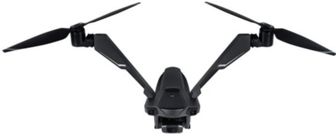
Figure 29. V-Coptr Falcon by Zero Zero Robotics with two tilting rotors [39] .
