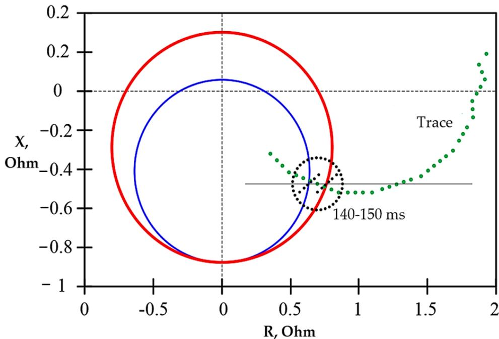
**Figure 4.** Estimation of damage detection time.
