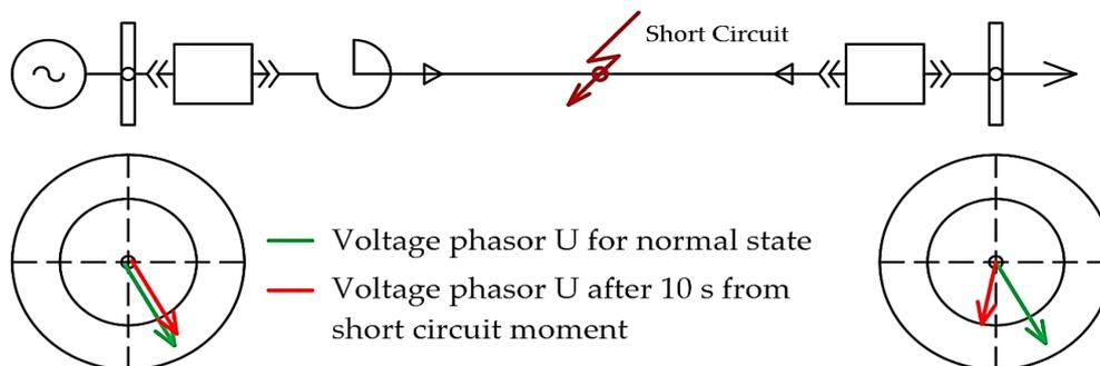
**Figure 1.** Change of voltage vectors in case of a short circuit on the line.
