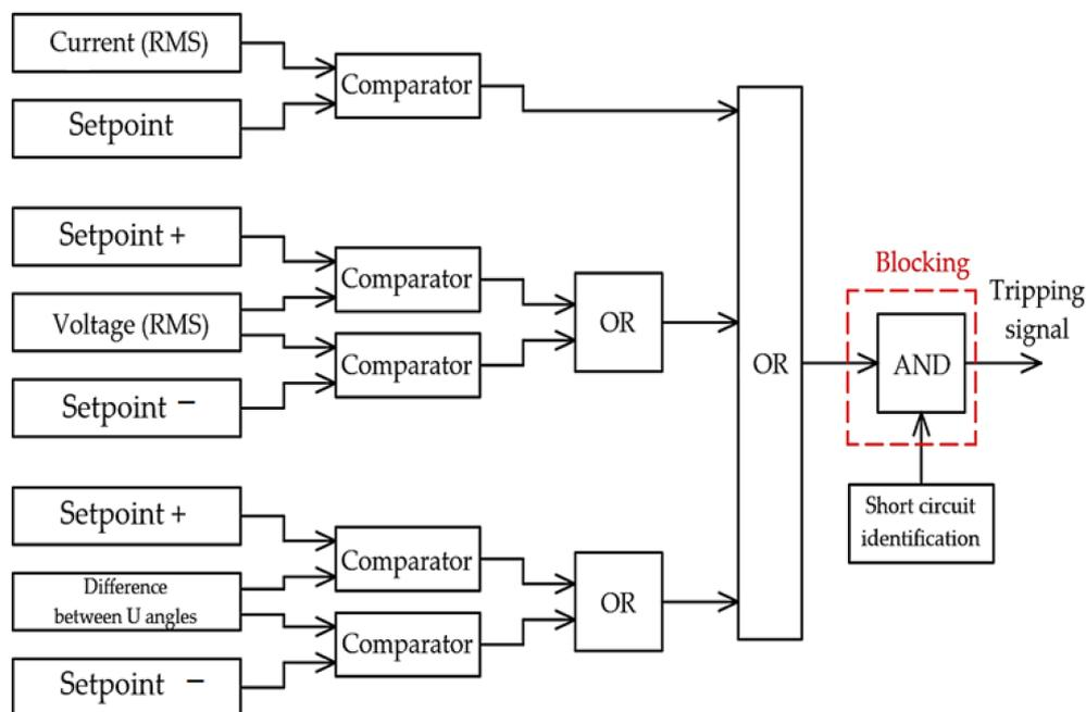
**Figure 2.** Block diagram of the use of voltage vectors to implement the current protection blocking function.
