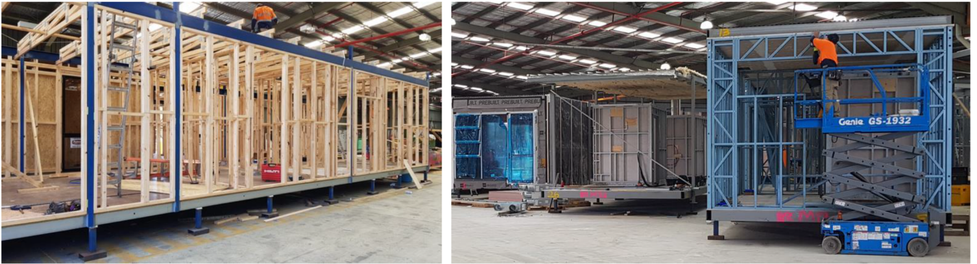
Figure 1. A steel modular unit with softwood wall frames ( left ) and a steel corner supported modular unit with a cold formed light-gauge steel wall frame ( right ), showing various materials used in prefabricated construction.
