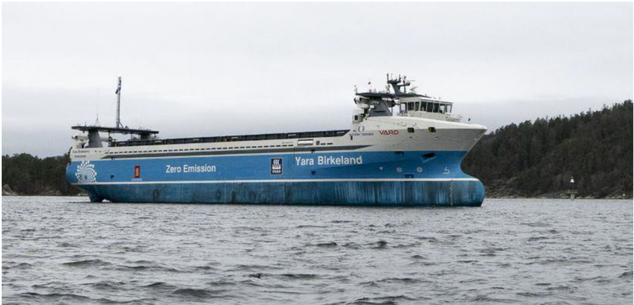
Figure 14. Yara Birkeland, the first fully electric and autonomous container ship [29] .
